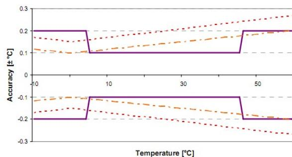
The following figure illustrates the accuracies of the BeanDevice® ONE-T High accuracy version and DIN A and DIN Y (1/3 DIN B) platinum sensors.
