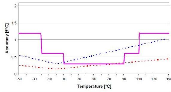
The figure above illustrates the accuracies of the BeanDevice® ONE-T standard accuracy version and DIN A and DIN B platinum sensors.
