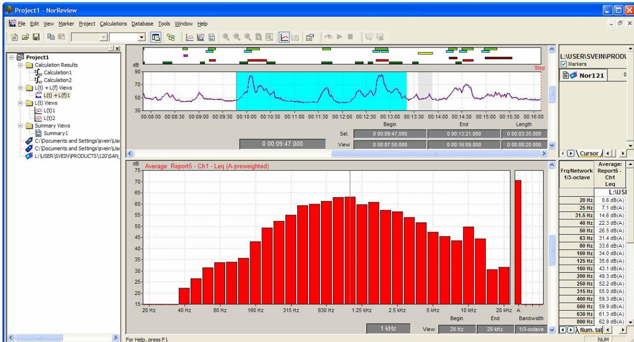
The split display showing a L(t) View (above) and a L(f) View (below) for evaluation of the frequency content at specific points or time-areas are of interest.
