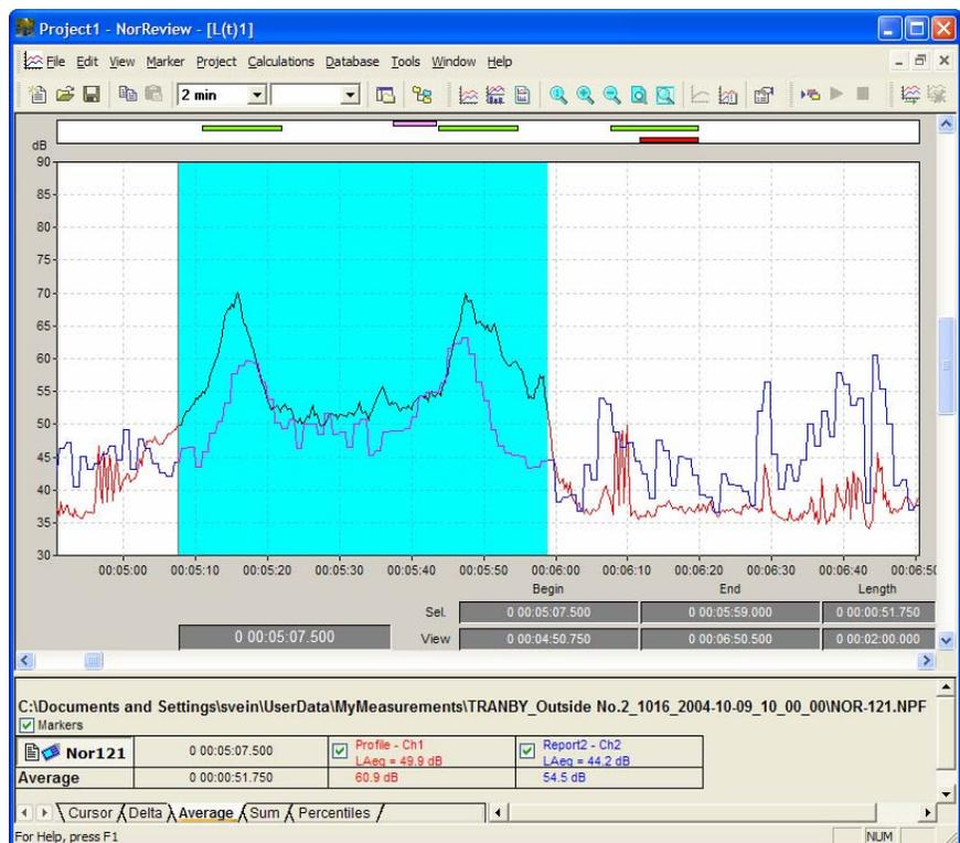
The Quick-Calc feature rapidly calculates levels from cursor-selected areas of the Level vs. Time measurement
