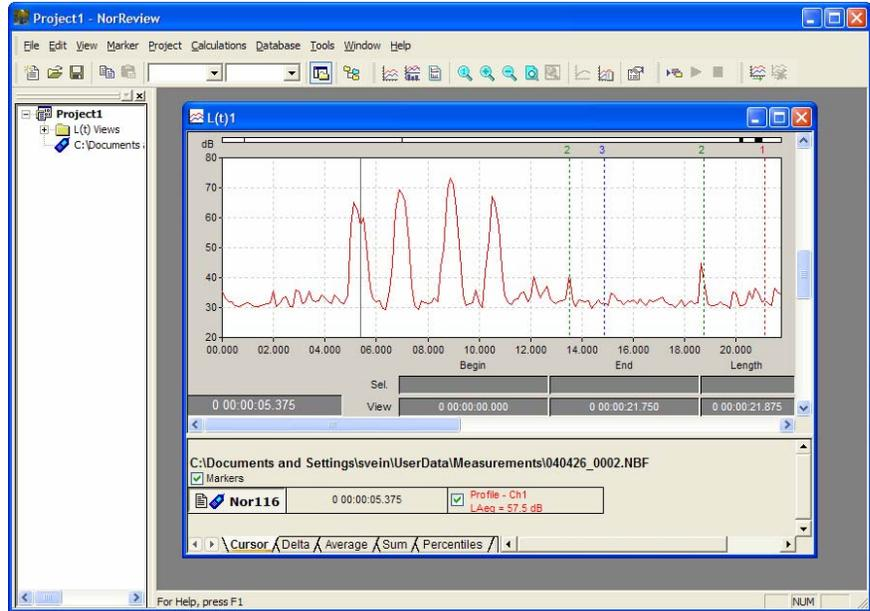
Automatically generated L(t) View of the initial measurement file dropped into the workspace section on the left-hand side
