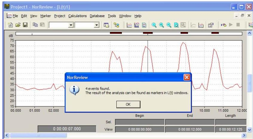
The Event Analysis inserts new markers along the x-axis where the pre-defined thresholds are met.
