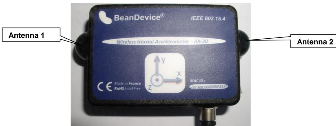
Figure 4: Antenna position on the BeanDevice AX-3D
