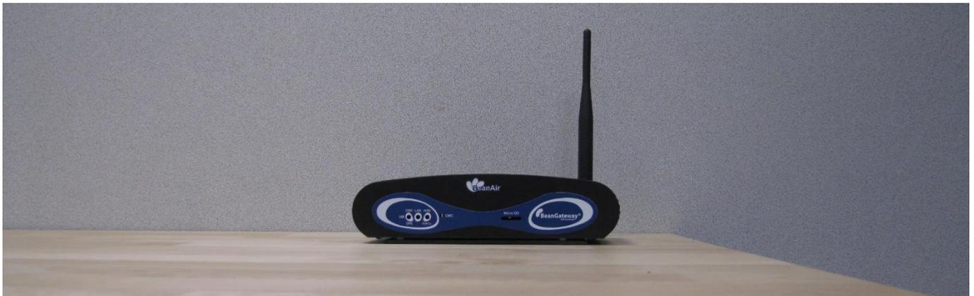
If your WSN is deployed on the same floor, a horizontal position of the antenna will decrease the RF signal.
