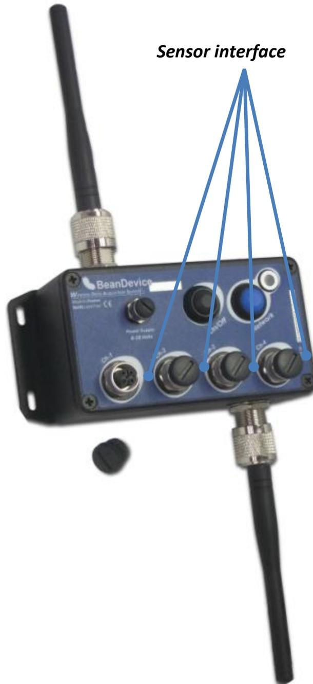
*Figure 9: M12 socket location the BeanDevice®*
