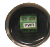
Internal View - 2 pin Terminal Block
